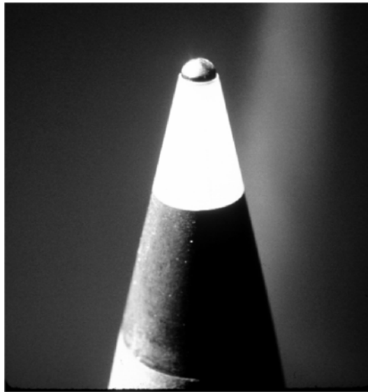
Figure 1: Nose tip probe biased at a DC voltage (typically, +5 V) for electron collection
